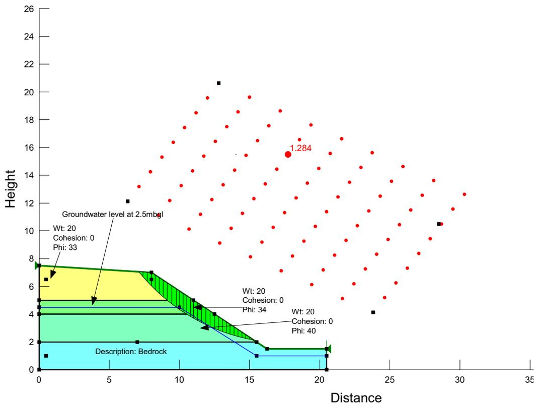
**Figure 4.1 Slope Stability Analysis for Open Cut Excavation (drained)**
