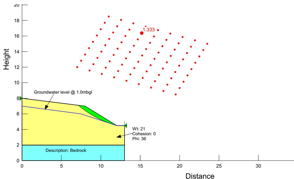
**Figure 6.1 Slope Stability Analysis for Open Cut Excavation (drained)**
