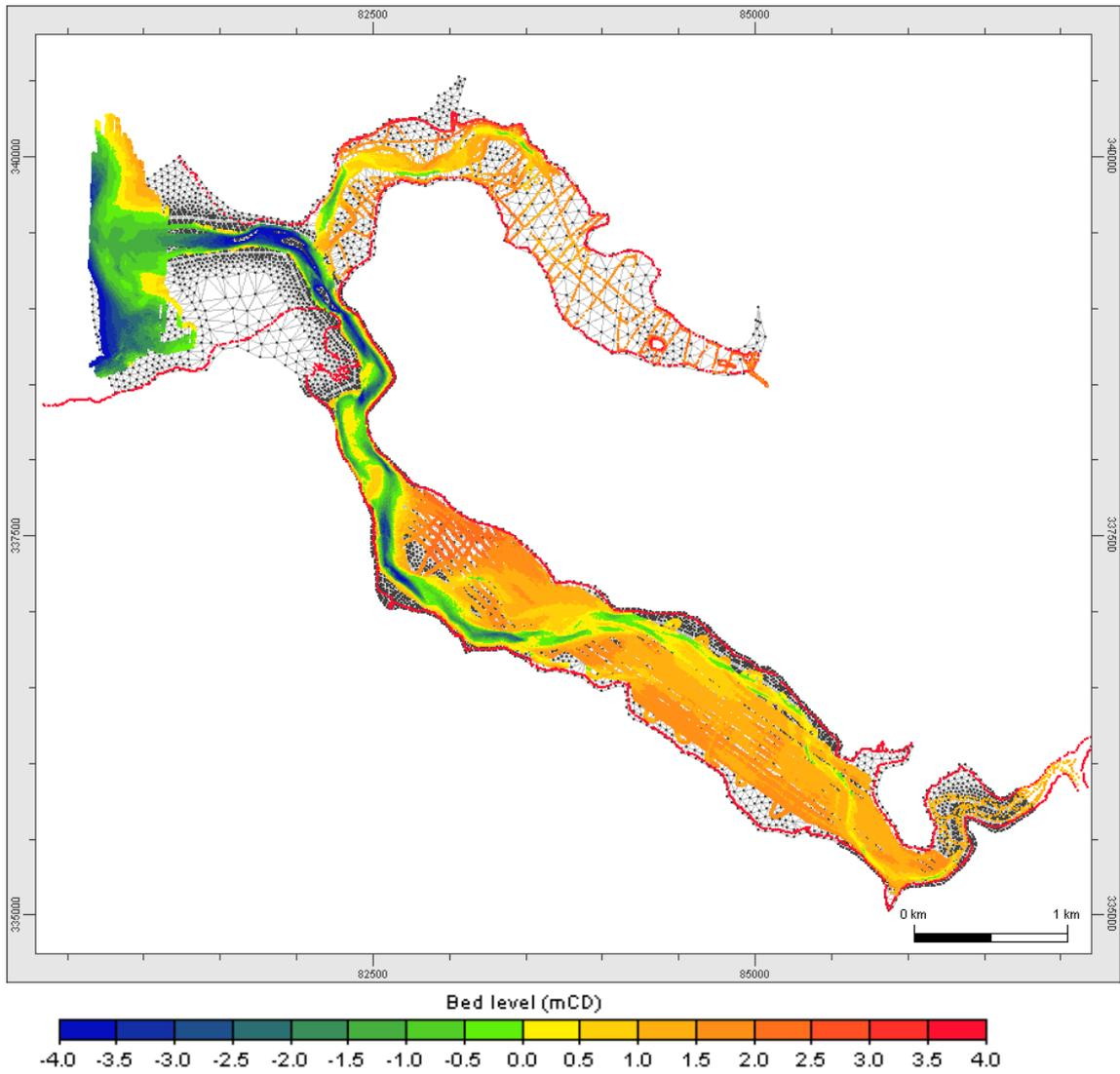
**Figure 1** Model mesh and bathymetric data coverage
