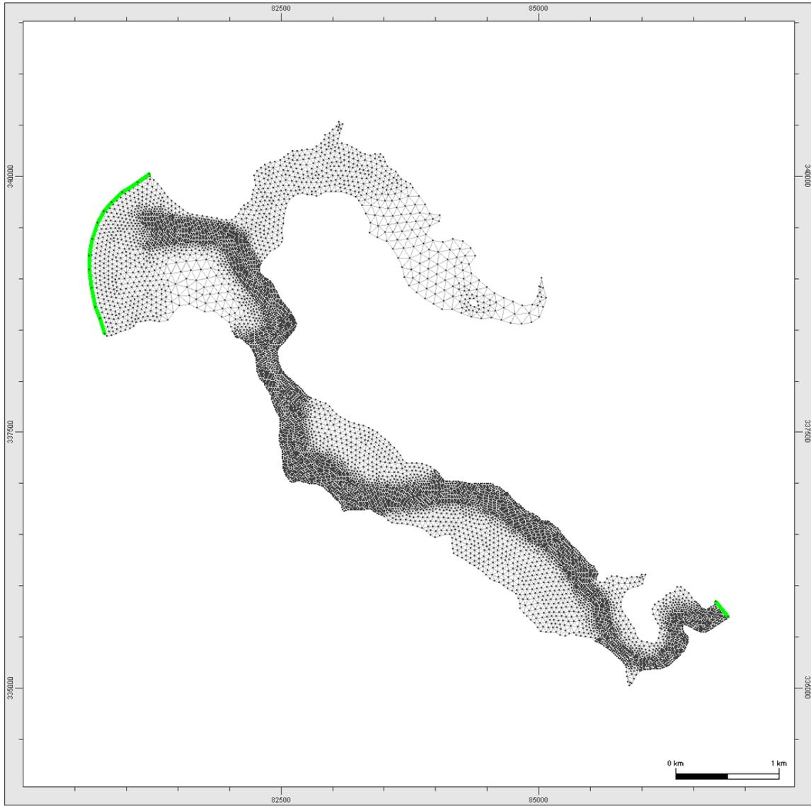
**Figure 4** Model mesh with location of the open boundaries (in green)
