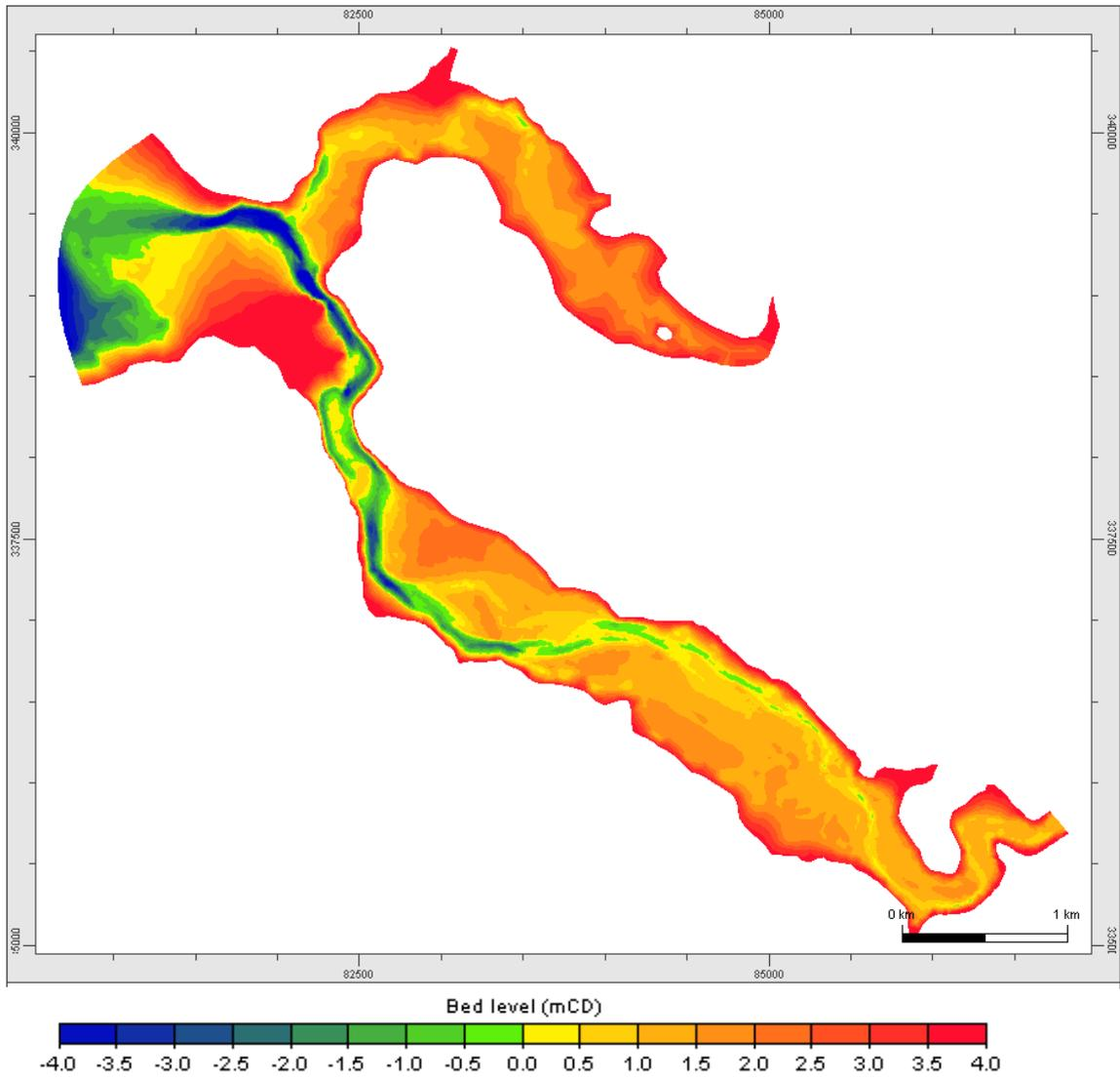
**Figure 5** Baseline model bathymetry
