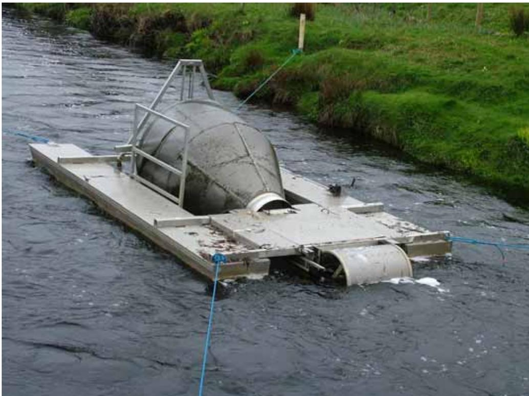
**Floating rotary screw trap Glenamoy River 2009**
