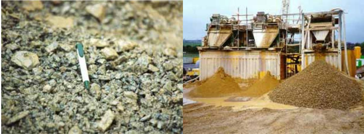
**Figure 3.1 Typical Rock Cuttings and Materials Separation Plant from Tunnelling Process**
